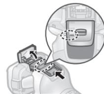
Press and hold the top knob (a) and slide the trimmer handle down to lower the trimmer.
