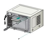
Mount the Top Duct [B] and the Left Duct [C] to the oven.
