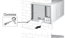
Depending upon the location of the AC outlet, route the AC cord to either the left or right side while installing the front grille.
