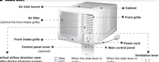
Vertical airflow direction vane (Airflow direction adjustment up-down). The vertical airflow direction vane is controlled by positioning the vane to discharge the air upwards, downwards, or straight out.
